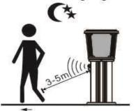
Step3: With PIR motion sensor function the whole night, when people approach, the light will turn to 200 lumens bright light and delay 30S.
