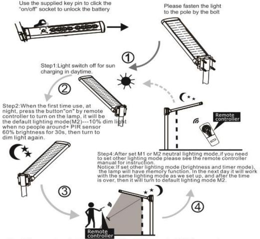
Step3:Use remote controller to choose M1 or M2 two neutral lighting mode M1(15%+PIR): 15% dim light when no people around+ PIR sensor 60% brightness for 30s, then turn to dim light again.
